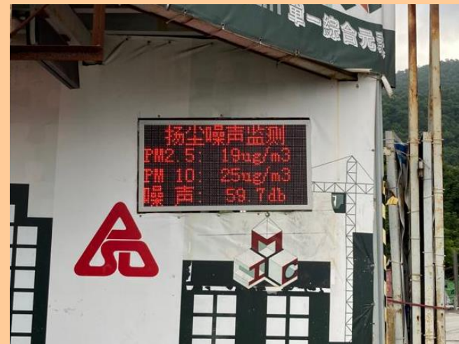
Real time monitoring PM10, PM2.5 and sound level
