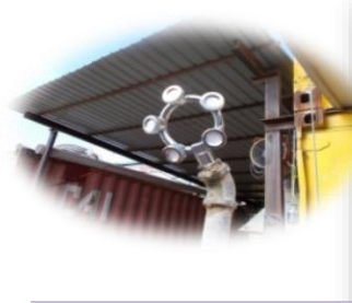
Reuse of waste metal as dust suppression facilities
